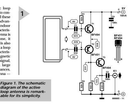
possibly even easier. Assuming that the dimensions of the window frame are 1 by 1.5 metres, you should wind two to four loops of insulated hook-up wire around small nails located at the corners of the frame. The core diameter of the wire is not particularly important. Be sure not to use a metallic window frame, since the antenna will not work at all with a metallic frame.
